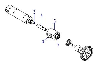
a) optional: explosion protected stainless steel sensor for speed measurement
